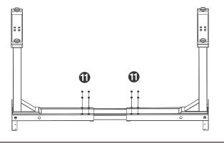
Double-check that the base is centered on the underside of the desktop and is located where I. you want it. Also, double-check that the included wood screws are not too long for your desktop and screwed all the way in.
