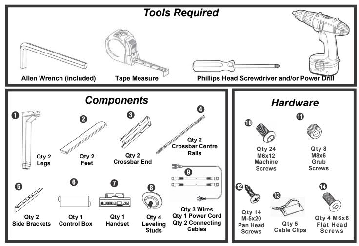
Please count all pieces before disposing of any carton or packing materials. Use a padded or carpeted area for assembly to avoid damage. For ease and safety, we recommend two people for assembly
