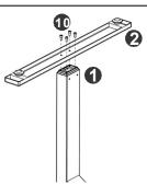
**G.** Your desktop may or may not be pre-drilled. Please check both sides of the desktop before placing the desk base on it for pre-drilling! Carefully place the upside down desk base on the underside of the desktop.
